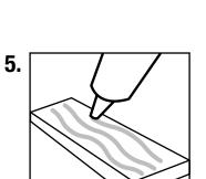
Use "Liquid Nail" or "PL Adhesive". Apply a generous amount to the back of the splash.
