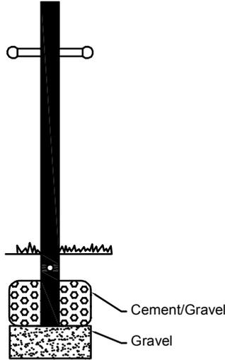
Dig a hole 12"- 15" in diameter to the depth shown in the diagram to the left. Consult local codes.
