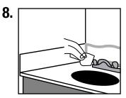
With a caulk edging tool, run it across the seams to clear away excess silicone & caulk (this technique will leave a clean line of silicone & caulk over the seams).
