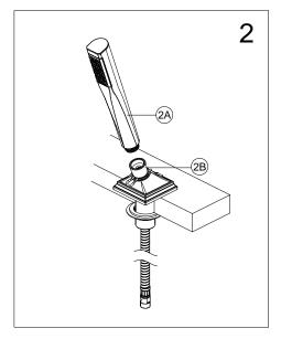
Connect hand held shower (2A) into the end of coiled hose (2B) by turning metal hose fitting clockwise. Hand tighten.
