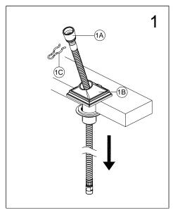
Insert coiled spray hose (1A) onto spray flange (1B). Restrain coiled spray hose (1A) with clip (1C), so that the coiled spray hose can't fall into spray flange and not to pull out.
