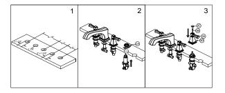
4.Mount spray support assembly. Place spray support assembly (4A) through mounting hole in deck. Secure spout body with rubber washer, metal washer and nut. Tighten nut securely with wrench
