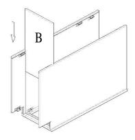
Slide the Back panel into the grooves in the side panels and attach the male clips to the back panel. There're three clips on the left side and three clips on the right side. Each male clip will need 2 small screws(I).
