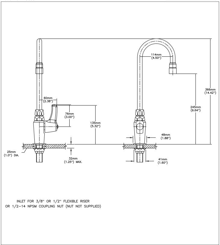
Delta reserves the right (1) to make changes to specifications and materials, and (2) to change or discontinue models, both without notice or obligation. Dimensions are for reference. Measurement may vary plus or minus 6mm(0.25"). Mounting locations are suggested only. Check with local codes for requirements in your area. This spec was produced May 27, 2021.
