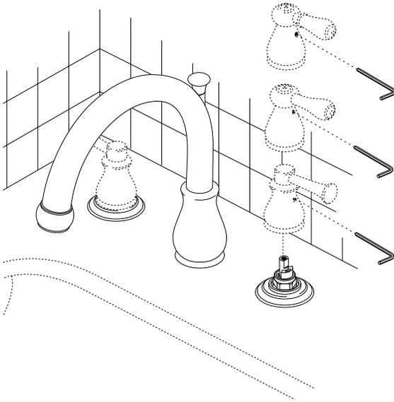
Install handles. **Be sure glide ring (1) is properly seated in bottom of handle before installing.** If either handle does not rotate in the correct direction, do the following:
