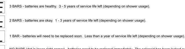
NO BARS (dot in lower-right corner) - batteries need to be replaced immediately. The solenoid has been locked out and will not fire until batteries have been replenished.
