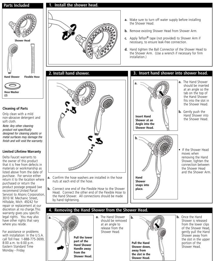
WARNING: Plumbing Codes require that shower heads and hand showers provide a small but continuous flow of water (trickle) when in "PAUSE" mode. Because of this continuous flow, in certain circumstances pressure variations in the water line and/or changes in the position of shower temperature control handle while in "PAUSE" mode could result in dramatic changes to the temperature of the water when the shower head or hand shower is returned to the "ON" position.
