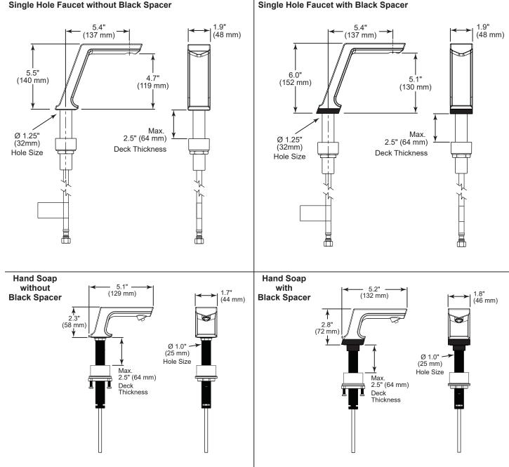
NOTICE Dimensions are for reference only. Measurements may vary ± 0.25" (6 mm). Max. flow rates are at 60 psi (414 kPa). WaterSense® is a registered trademark of the U.S. Environmental Protection Agency.
