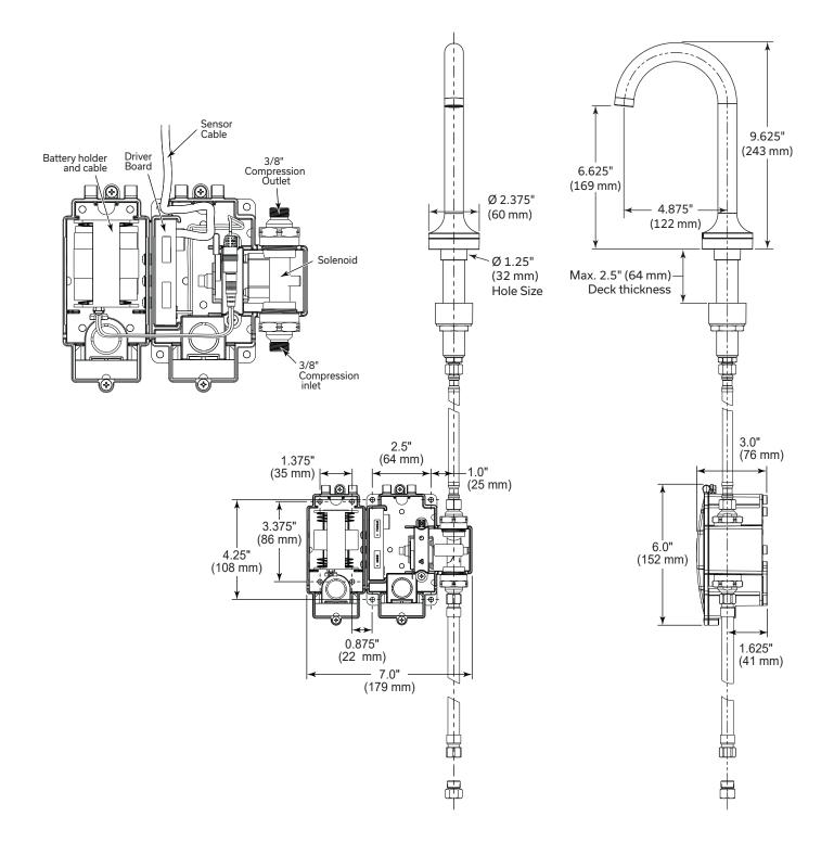
**NOTICE** Dimensions are for reference only. Measurements may vary ± 0.25" (6 mm). Max. flow rates are at 60 psi (414 kPa). **WaterSense**<sup>®</sup> is a registered trademark of the U.S. Environmental Protection Agency.
