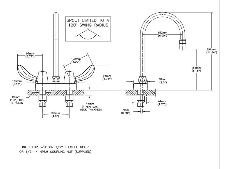
Delta reserves the right (1) to make changes to specifications and materials, and (2) to change or discontinue models, both without notice or obligation. Dimensions are for reference. Measurement may vary plus or minus 6mm(0.25"). Mounting locations are suggested only. Check with local codes for requirements in your area. This spec was produced November 01, 2011.
