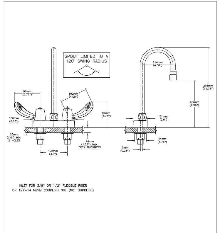
Delta reserves the right (1) to make changes to specifications and materials, and (2) to change or discontinue models, both without notice or obligation. Dimensions are for reference. Measurement may vary plus or minus 6mm(0.25"). Mounting locations are suggested only. Check with local codes for requirements in your area. This spec was produced November 29, 2016.
