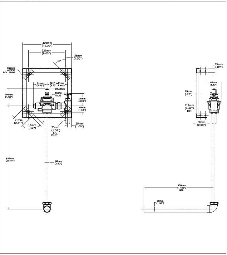
Delta reserves the right (1) to make changes to specifications and materials, and (2) to change or discontinue models, both without notice or obligation. Dimensions are for reference. Measurement may vary plus or minus 6mm(0.25"). Mounting locations are suggested only. Check with local codes for requirements in your area. This spec was produced December 20, 2016.
