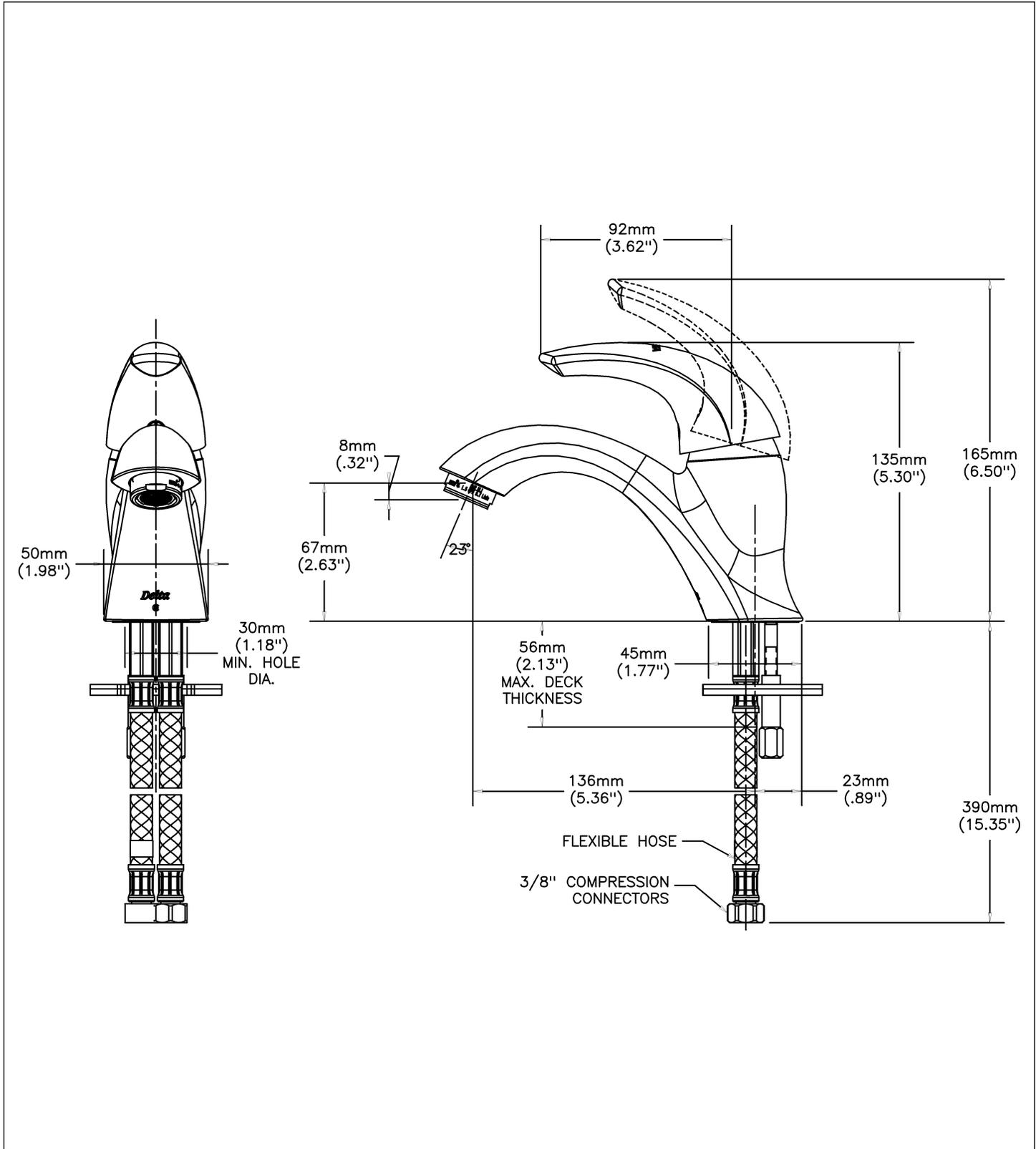
Delta reserves the right (1) to make changes to specifications and materials, and (2) to change or discontinue models, both without notice or obligation. Dimensions are for reference. Measurement may vary plus or minus 6mm(0.25"). Mounting locations are suggested only. Check with local codes for requirements in your area. This spec was produced May 04, 2021.
