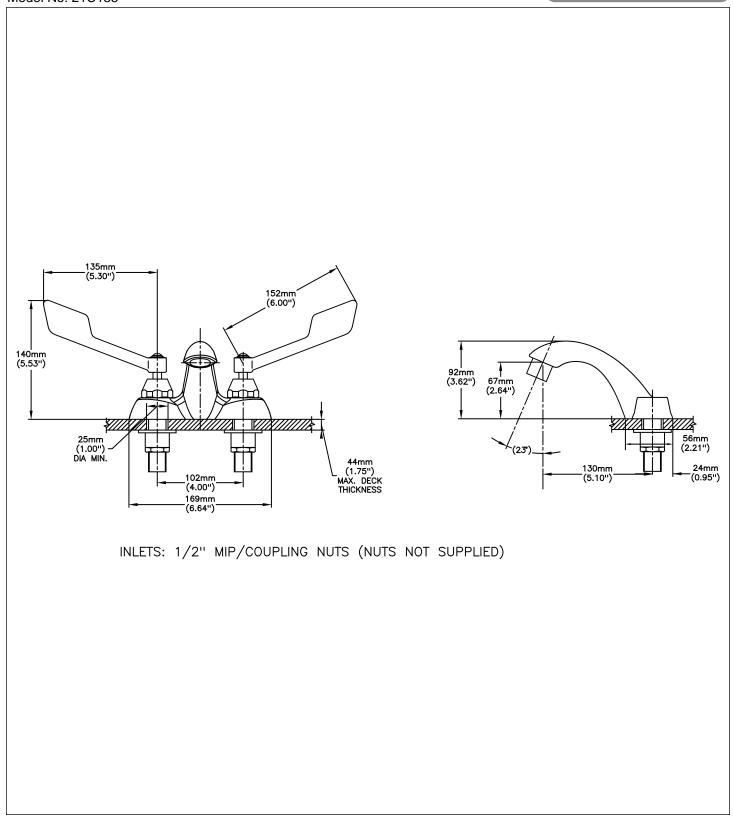
Delta reserves the right (1) to make changes to specifications and materials, and (2) to change or discontinue models, both without notice or obligation. Dimensions are for reference. Measurement may vary plus or minus 6mm(0.25"). Mounting locations are suggested only. Check with local codes for requirements in your area. This spec was produced June 21, 2021.
