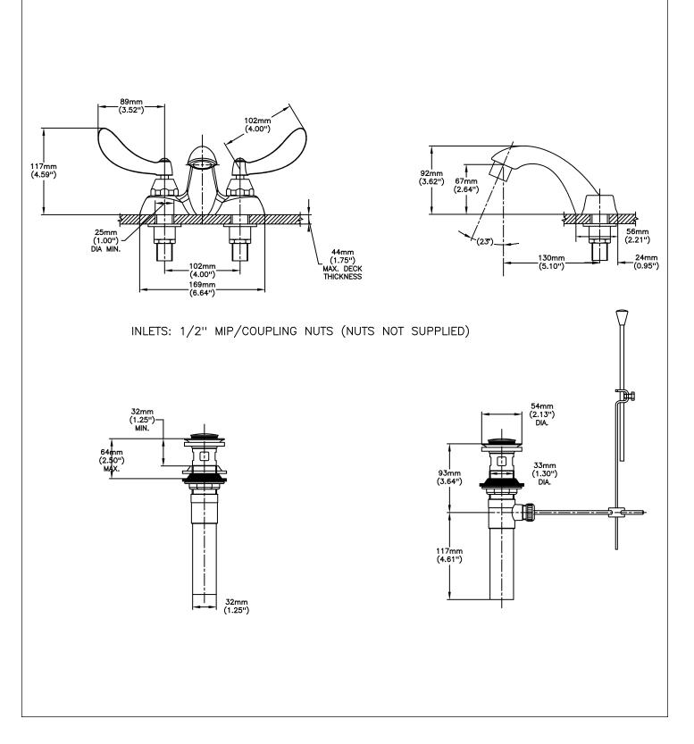
Delta reserves the right (1) to make changes to specifications and materials, and (2) to change or discontinue models, both without notice or obligation. Dimensions are for reference. Measurement may vary plus or minus 6mm(0.25"). Mounting locations are suggested only. Check with local codes for requirements in your area. This spec was produced June 17, 2021.
