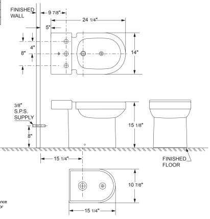
IMPORTANT: Dimensions of fixtures are nominal and may vary within the range of tolerance established by ASME Standard A112.19.2. These measurements are subject to change or cancellation. No responsibility is assumed for use of superseded or voided pages.
