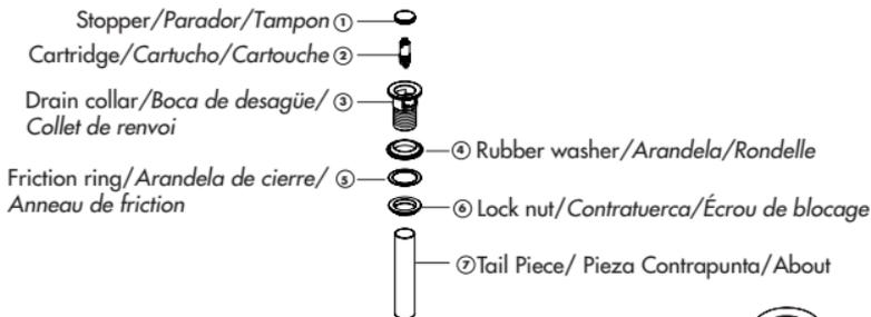
1. Remove rubber washer (4), friction ring (5) and lock nut (6) from the drain assembly.
