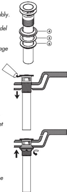
**For drain cartridge replacement or cleaning**
