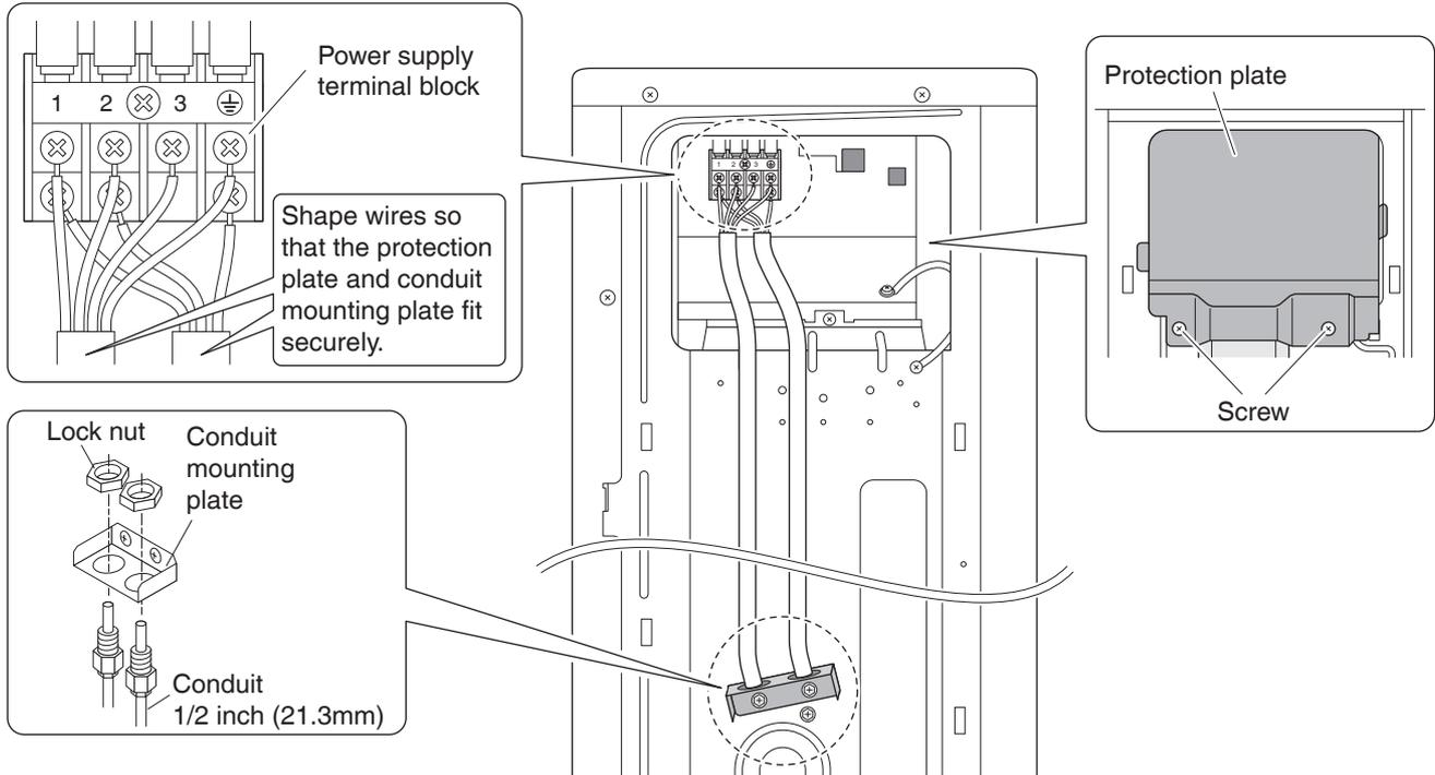
Observe the notes mentioned following when wiring to the power supply terminal board.
