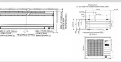
Wall height on air outlet side = Less than 47-1/4"
