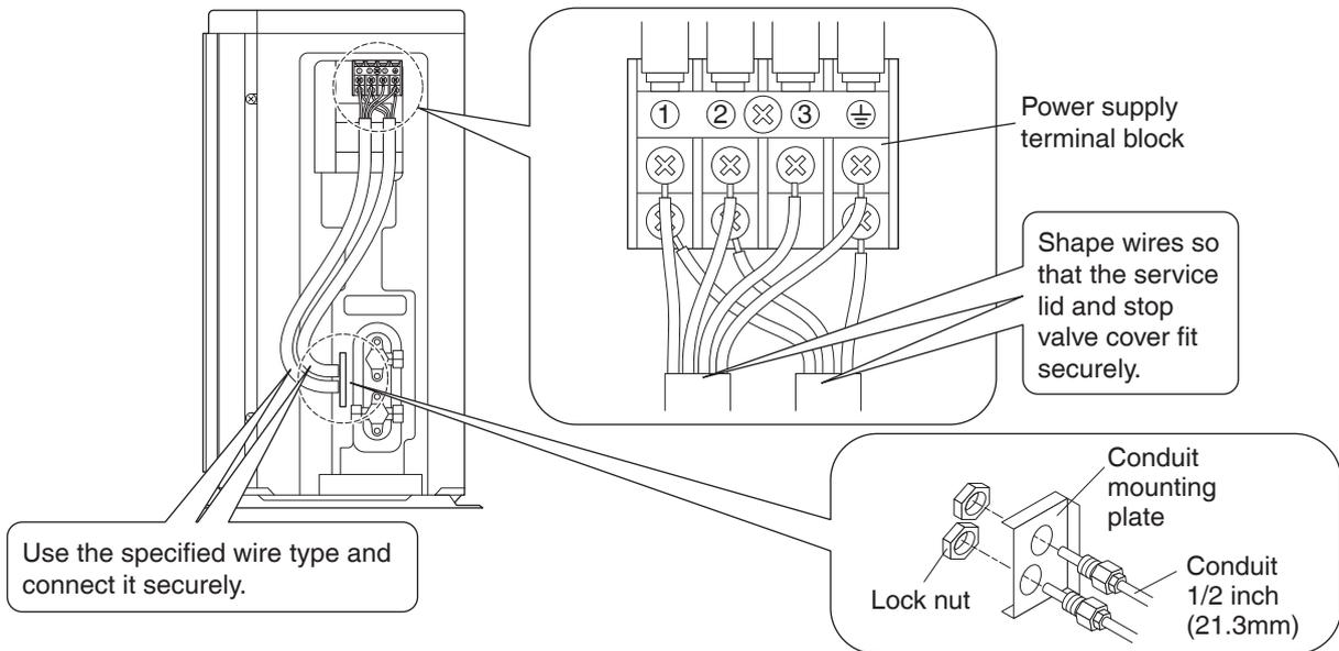
Observe the notes mentioned following when wiring to the power supply terminal block.
