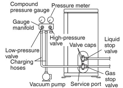
1) Connect projection side of charging hose (which comes from gauge manifold) to gas stop valve's service port.
