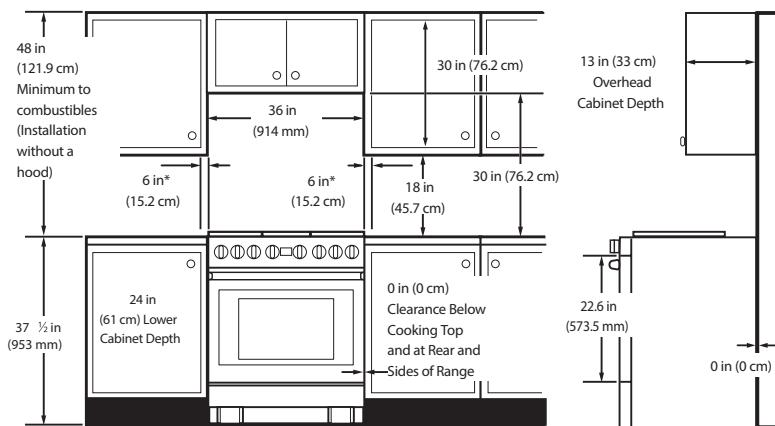
\* Side clearance above cooking surface to any objects, i.e., wall.
