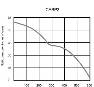
Airflow CFM (Cubic feet/minute)
