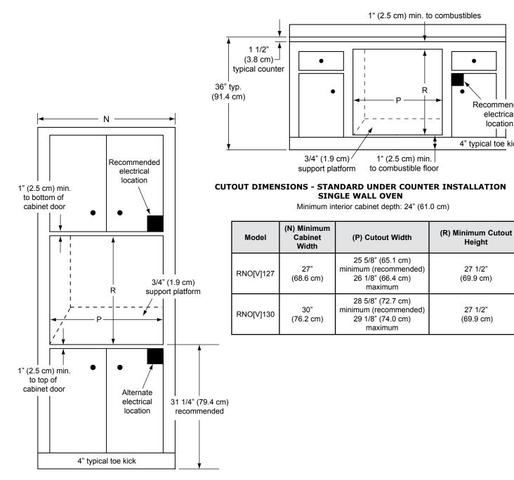
**CUTOUT DIMENSIONS - STANDARD WALL INSTALLATION** SINGLE WALL OVEN
