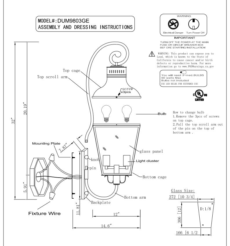
After securing fixture to wall, it is recommended that the gap between the wall and backplate be sealed on top and both sides with a good quality waterproof caulk or silicone sealant (not included)
