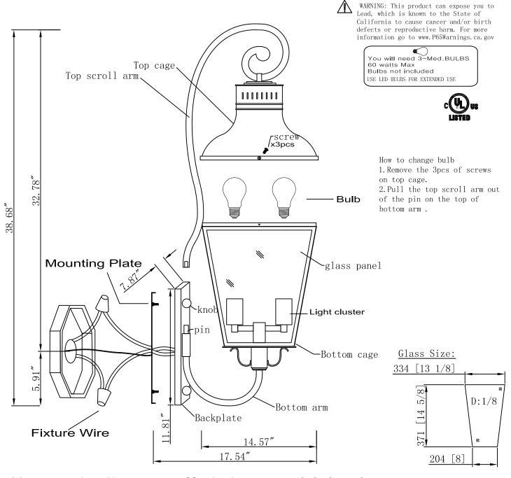
After securing fixture to wall, it is recommended that the gap between the wall and backplate be sealed on top and both sides with a good quality waterproof caulk or silicone sealant (not included)
