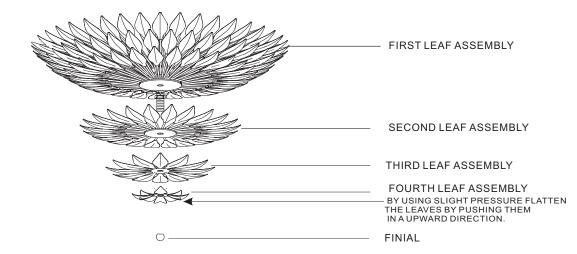
NOTICE: FOR REPLACING THE BULB, PLEASE UNSCREW THE LEAF ASSEMBLY AS SHOWN ABOVE
