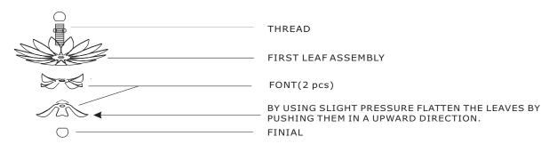
ASSEMBLE THESE PARTS TO THE BOTTOM
