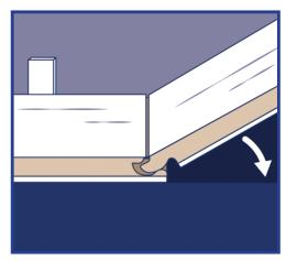
Step 2: Lock short end of flooring by inserting tongue into groove at an angle and drop in place. At end of the row, measure and cut the flooring to complete the row. Install the cut edge closest to the wall.
