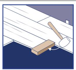
Step 7: Tap end of flooring with hammer and tapping block to lock ends of flooring together.
