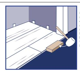
Step 1: Undercut space under door jamb to allow flooring to slide freely. Tap long edge with hammer and tapping block to lock long edge.
