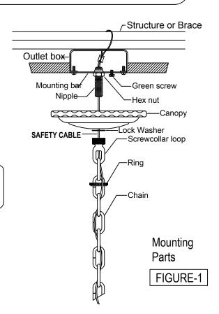
3. Open the end links of the chain and attach the chain to the screw collar loop. Hang the fixture on the chain at the desired height. Remove the excess chain close all links. Unscrew the threaded ring from the screw collar loop. Allow the ring and canopy to slide down the chain to the top of the fixture.
