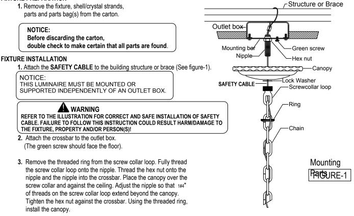
4. Open the end links of the chain and attach the chain to the screw collar loop. Hang the fixture on the chain at the desired height. Remove the excess chain close all links. Unscrew the threaded ring from the screw collar loop. Allow the ring and canopy to slide down the chain to the top of the fixture.
