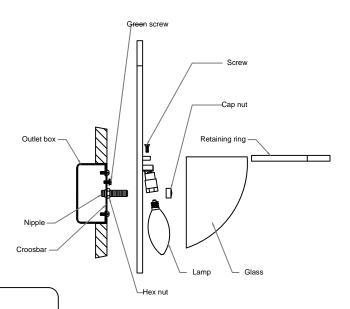
**4.** Fasten the white fixture lead to the white wire in the outlet box. Fasten the wires together with an approved fastener (wire nut). Starting about 1" below the fastener, tightly wrap the connection with electrical tape so that the connections seals the end of the fastener.
