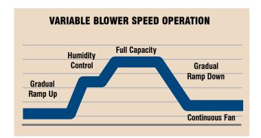
Gradual ramp up and down of the variable speed motor significantly reduces sound.
