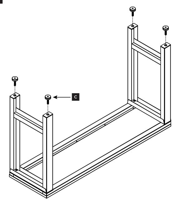
\*Maximum height extension for adjustable feet is 1.5 in. \*Please note location of predrilled holes on each part.
