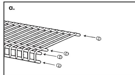
**2** a. Lightly draw a level line at desired shelf location the exact length of shelf. Measure and mark a wall clip location 2" from each end of shelf. Measure and mark all remaining clips as shown below. For cut shelves in other sizes, install a wall clip 2" from each end of shelf and space remaining wall clips at even intervals between end wall clips. **Never install wall clips more than 12" apart.**
