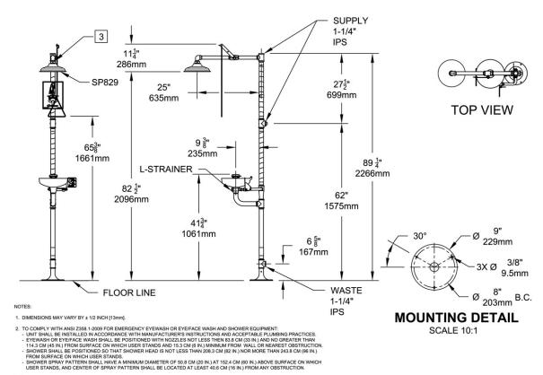
3. DO NOT USE REGULAR PIPE SEALANT. IF NECESSARY USE DOW CORNING 832 SEALANT PLACING 5 SMALL BEADS ON THE MALE THREADS, JUST ABOVE THE FIRST THREAD.
