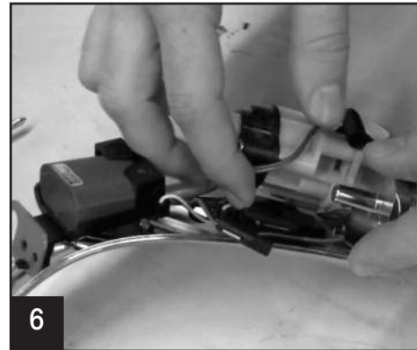
6 Position new electronics module into faucet.
