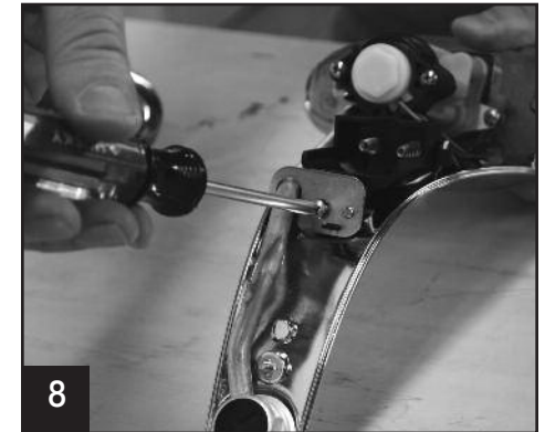
8 Resecure module with mounting plate and screw.
