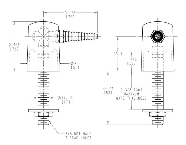
DIMENSIONS ARE IN INCHES AND [MILLIMETERS].
