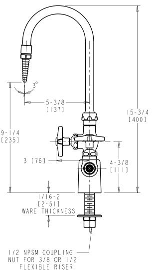
DIMENSIONS ARE IN INCHES AND [MILLIMETERS].
