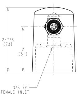
DIMENSIONS ARE IN INCHES AND [MILLIMETERS].
