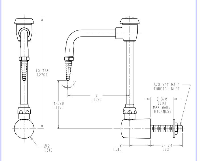
DIMENSIONS ARE IN INCHES AND [MILLIMETERS].
