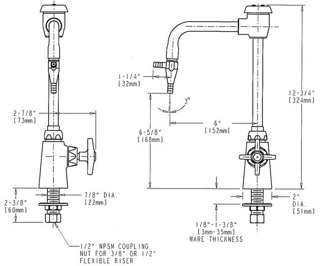
DECK MOUNTED SINGLE WATER INLET FITTING GN2BVB RIGID/SWING VACUUM BREAKER SPOUT
