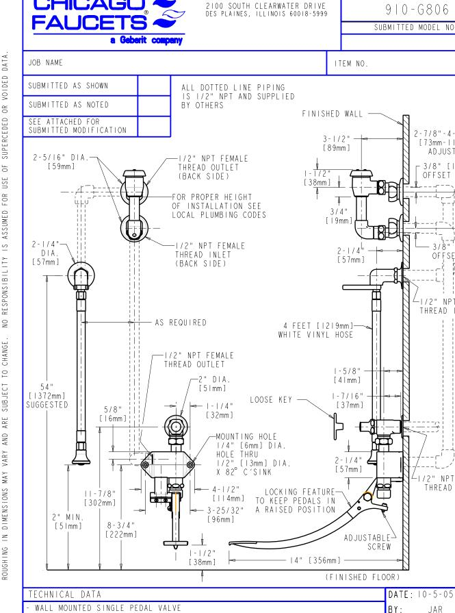
FITTING NO. 910-6806 SUBMITTED MODEL NO 2-7/8"-4-3/8"-[73mm-|||mm] ADJUSTABLE 3/8" [I0mm] OFFSET 3/8"<sup>!</sup>[|Omm] OFFSET 1/2" NPT FEMALE THREAD INLET 1/2" NPT FEMALE THREAD INLET
