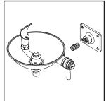
(2) Apply Teflon tape on both thread ends of brass nipple, thread and tighten brass nipple to wall bracket. Thread and tighten drinking fountain to brass nipple. Ensure the drinking fountain is in level position.
