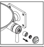
(5) The self-close basin faucet was preset @60 PSI to shut off water, different water pressure might affect the faucet and cause it not to function properly, if need be, remove the handle cap, sleeve and Celcon Samson nut.
