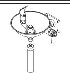
(3) Apply Teflon tape to the thread end of drain adapter. Thread and tighten drain adapter to the drink fountain.
