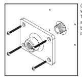
(1) The 3/8" pipe thread nipple must be kept with a length of 1/2" from finished wall. Apply Teflon tape at the thread end of pipe nipple stretch out from finished wall. Thread wall bracket to 3/8" pipe nipple and secure the wall bracket with supplied four screws.
