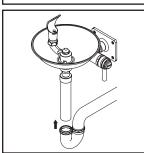
(4) Attach drain adapter to the P-trap.
