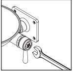
(6) Use wrench to adjust brass square nut, turn counterclockwise to tighten the cartridge and turn it clockwise to loosen the cartridge until the faucet functions properly then proceed to tighten the cartridge 90° more before reassembling the Celcon Samson nut, sleeve, and handle cap back in place.
