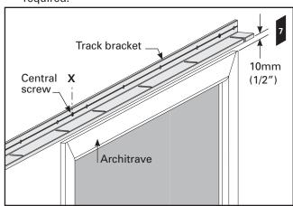
Level track bracket by pivoting around central screw. Lock in place with two outer screws.
