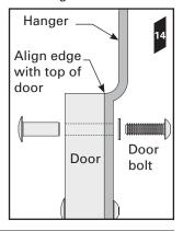
If you are installing SofStop, follow steps 20-21, Page 4 to fit the activator to the top of the door.
