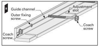
Slide track onto the bracket and immediately fix the track to the bracket with bolts and washers to ensure track does not fall off.
