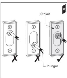
13. The striker allows 2.5mm (3/32") of adjustment in each direction when the striker face plate is fitted in the centre of the striker body.
