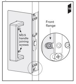
17. Use the ball end of the CL400 Allen key to tighten the 2x handle joining screws. Use the other end of the Allen key to firmly tighten the screws.
