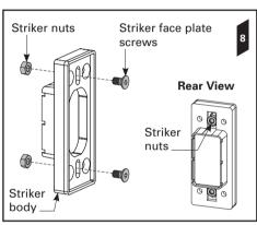
9. Insert the striker body, with the striker face plate screws and the striker nuts attached, into the cut out in the closing
