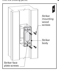
**10**. Remove the striker face plate screws. The striker nuts are now trapped in position.
