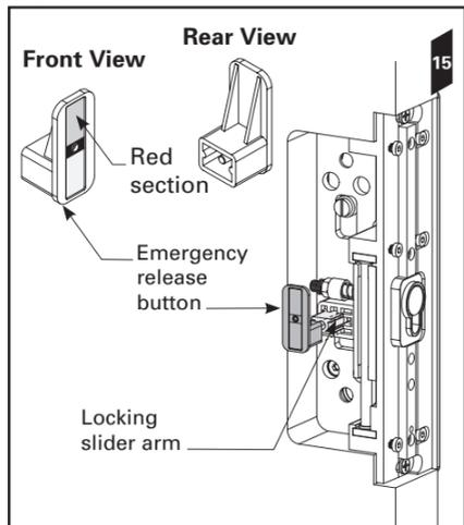
**Fitting the Remaining Side Handle and Face Plate**
