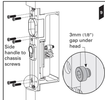
**10.** Fit the *privacy side handle* containing the snib button to the chassis as follows (if installing a snib/snib privacy handle install **ONE** of the side handles only):
