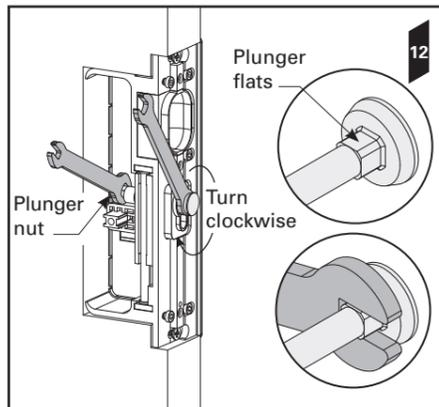
**13.** Continue to turn the spanner until there is no longer a gap between the spanner and the shroud face. Now turn the spanner **anti clockwise** half a turn. The plunger should now be adjusted correctly. Slide the doors closed to check that they latch. If the snib button is hard to push down or the plunger doesn't engage, adjust as necessary.
