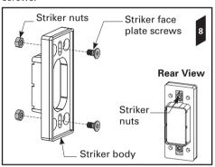
9. Insert the striker body, with the striker face plate screws and the striker nuts attached, into the cut out in the closing
