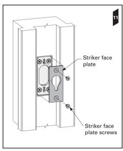
12. Close the door. When the striker is fitted correctly the magnet will draw the plunger forward. If this does not happen the striker is misaligned with the plunger (see below). If the alignment is correct, tighten the screws and skip to Step 14; otherwise continue to Step 13.
